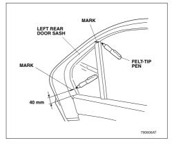
Temporarily position the two frame clips on the door sash aligning the end of the frame clips with the marks you made in step 4 and attach the pieces of masking tape as shown.
