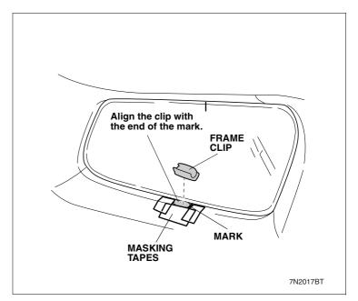
17. Apply primer to the parts of the left quarter sash enclosed with the masking tapes and let it dry thoroughly.
