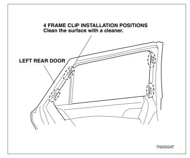
3. Using a felt-tip pen, make two marks in the positions shown.
