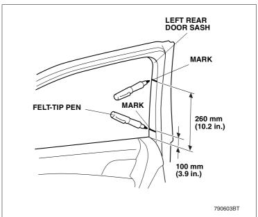
4. Using a felt-tip pen, make two marks in the positions shown.
