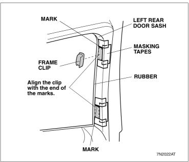
6. Temporarily position the frame clip on the left rear door sash aligning the end of the frame clip with the marks you made in step 4 and attach the pieces of masking tape as shown.
