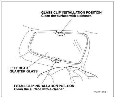
15. Using a felt-tip pen, make two marks in the positions shown.
