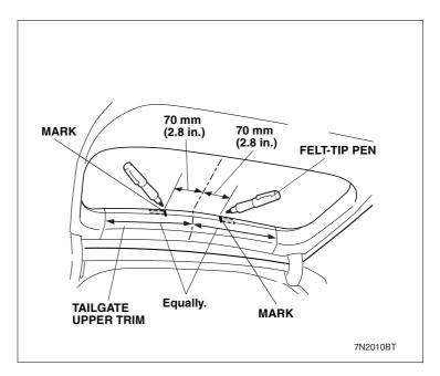
27. Temporarily position the frame clip on the tailgate upper trim aligning the end of the frame clip with the marks you made in step 26 and attach the pieces of masking tape as shown.
