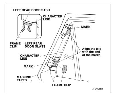
Apply primer to the parts of the door sash enclosed with the masking tapes and let it dry thoroughly.
