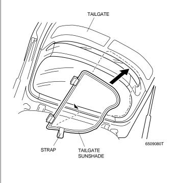
5. Install another tailgate sunshade aligning it with the tailgate. Join the two tailgate sunshades together with the two joint clips.
