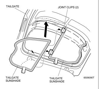
Secure the tailgate sunshades by inserting the two flat clips into the gap between the glass and trim.
