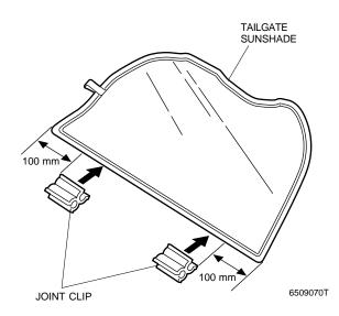
4. Install the tailgate sunshade aligning it with the tailgate.
